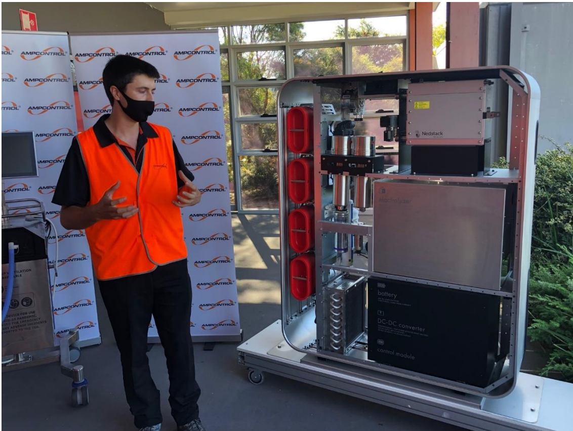
Hydrogen energy storage system for domestic and residential use developed with Ampcontrol (31 January 2022)
